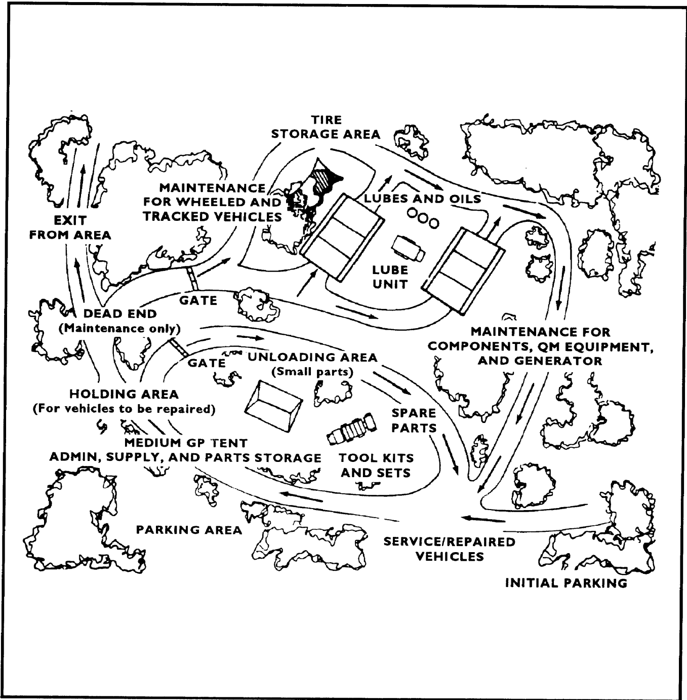
Figure 5-3. Sample maintenance section layout
